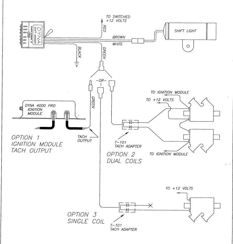
AUTO SHIFT CONFIGURATION USING STANDARD IGNITION WITH DRL—400 & DSM
